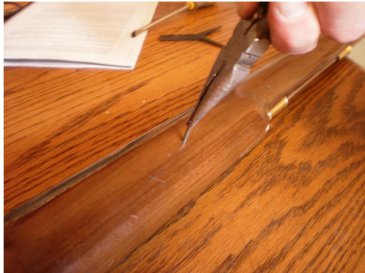
Remove pins with pliers or vise grips
