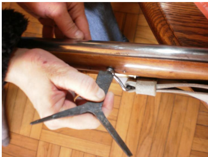
Remove the upper sling swivel and breech tang screws
